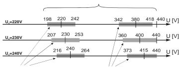
The voltage range U  $_{\text{L-N}}$ , for which the short-circuit current is calculated
