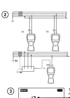
Connect test leads according to the drawing
